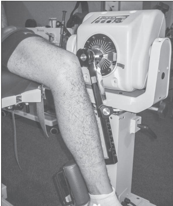
▲ Figure 4.26 Subject in an isokinetic dynamometer.
